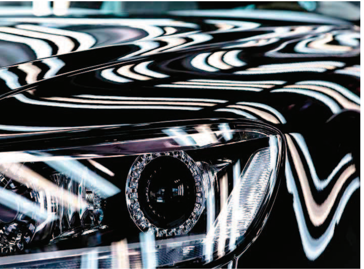
The surface control optics from OLIGO are installed in the light tunnel to create reflections that make defects on reflective surfaces more visible.
